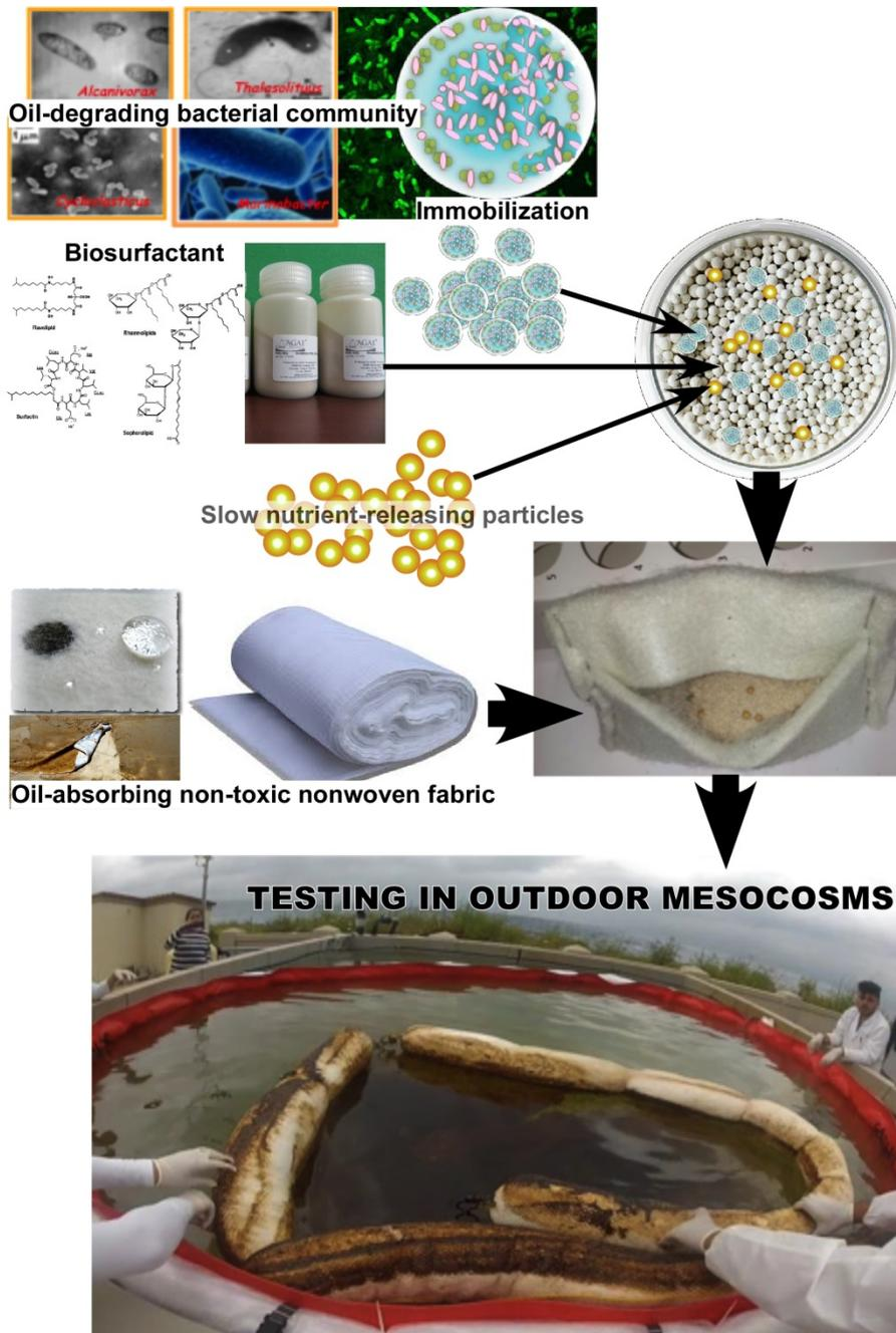
Figure 1 A schematic representation of the preparation of self-regenerating Bio-Boom oil-sorbent and subsequent testing in outdoor mesocosms.
