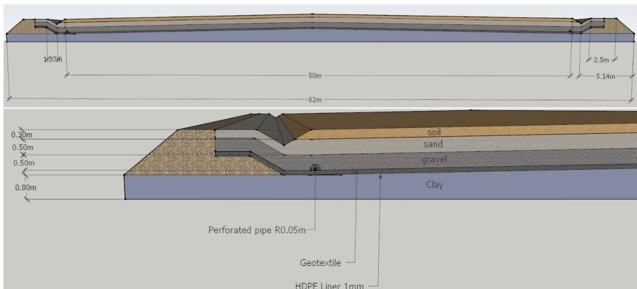
**Figure 1** Design details of Landfarming Units (top) overall diagram – width view and (bottom) berm details.
