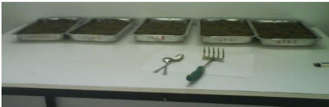
**Figure 2 Mesocosm biotreatability study of soil contaminated with petroleum hydrocarbons**
